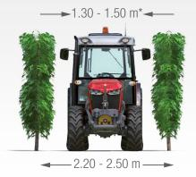
From 1.3m width, ideal for more open vineyards from 2.2-2.5m between the rows, with a slightly wider chassis with a more spacious cab for the operator.
