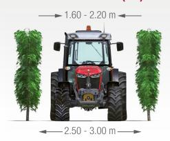
From 1.5m wide, ideal for hillside vineyards and alpine farms, offering a low centre of gravity and greater stability on slopes with a wider front and rear axle and a more spacious cab. Also ideal as a light utility tractor. Suitable for row widths from 3m.
